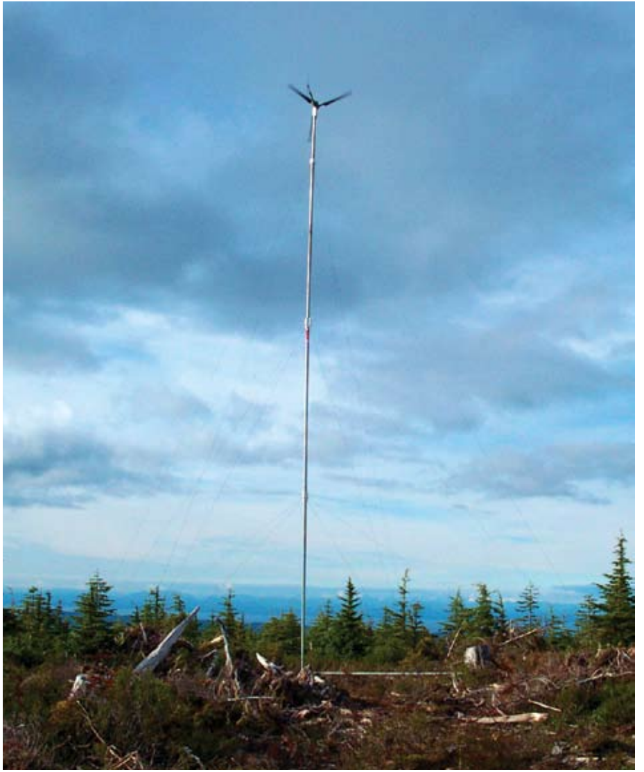
As wind speed increases with height, a tall tower is essential for greater wind output.
